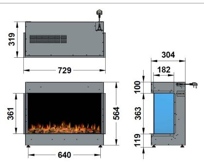
FRAME BUILD OUT DIMENSIONS (All dimensions are in millimetres)
