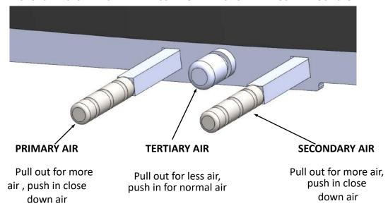
Air regulation, the three control levers perform differing tasks in regulating the combustion air on your appliance:
