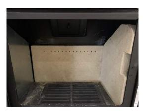
It is now possible to remove the top baffle brick by lifting up the left side and sliding it to the left then dropping it down.
