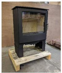
Right the stove and see if the legs are in the correct position; they should be inline with the front legs of the Churchill and have an even overhang where the legs meet the stove body. If not then loosen one leg at a time and adjust until satisfied.
