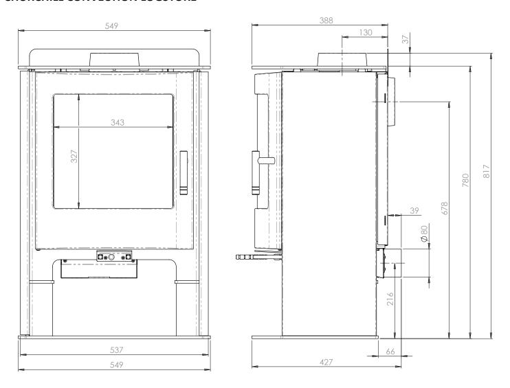
\*\* The additional, top flue rear convection panel (supplied loose within the stove) needs to be used when installing the stove 100mm from a combustible wall; this slots over the rear convection panel and provides additional radiant protection from the flue collar.
