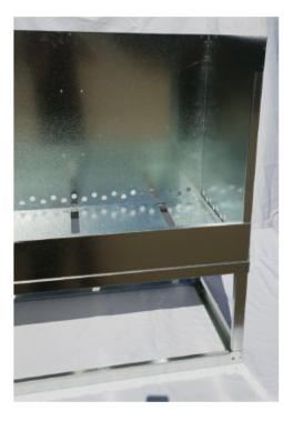
NOTE: When screwing 2 panels together through the existing holes, the screw should go through the larger hole first, then through the smaller hole, and cutting the thread in the smaller hole. I.e. some holes may screw from the inside, some from the outside.
