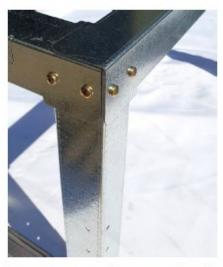
The completed assembled base, with 4 long rails joining the 2 Rectangle side frames:
