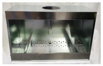
The top panel fits on, with the folds on the outside of all the other panels. Alternatively, it could be fitted on the inside of the side panels, so the holes are the same size.
