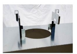
The brackets are fixed to the 8" inner casing is sealed into the top of the Zero Clerance box. And the the upper folded U-shaped hook is fixed to the 10" outer casing to keep it spaced 70mm off the ZCB. These can be fixed with self-tapping screws or rivets.
