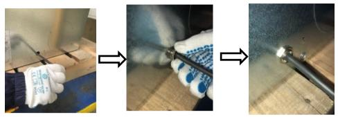
7. To install the thermostat, start by relieving the clips on the underside of the firebox, as seen bellow and placing the thermostat in position. Rotate it between the clips.
