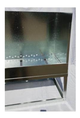
NOTE: When screwing 2 panels together through the existing holes, the screw should go through the larger hole first, then through the smaller hole, and cutting the thread in the smaller hole. I.e. some holes may screw from the inside, some from the outside.
