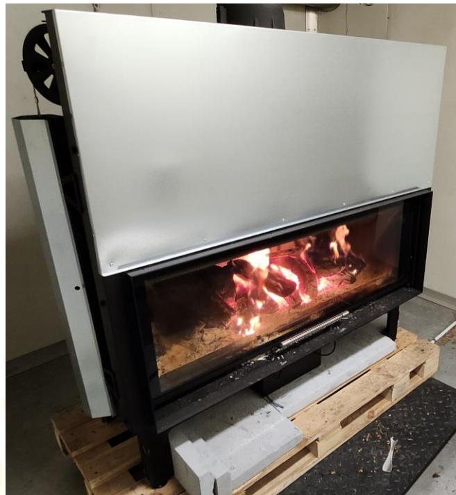
Figure 1: Appliance during testing.
