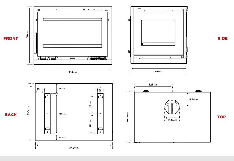
MATERIALS STEEL, CAST IRON KW OUTPUT 20 KW EFFICIENCY 62% AVERAGE I 67% LOW BURN EMISSIONS 0.6 G/KG HEATING CAPACITY 150 M2 - 230 M2\*
