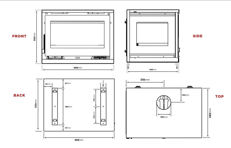
MATERIALSSTEEL, CAST IRONKW OUTPUT14.5 KWEFFICIENCY64% AVERAGE | 71% LOW BURNEMISSIONS0.7 G/KGHEATING CAPACITY100 M2 - 200 M2\*
