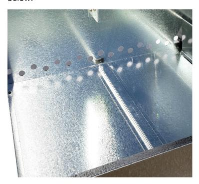
Step 6:Add the Heater support rails to the base. With 4 screws each.
