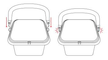
**3.** Rotate pram connectors. On the side of the basket, press the large round buttons then rotate the pram connectors to a vertical position as shown.
