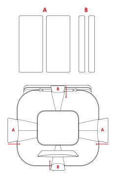
Attach the handle. Push the handle into slots on either side of basket until mechanism clicks in. To remove the handle from one side or both, press the oval button on the side you want to release and pull the handle out.
