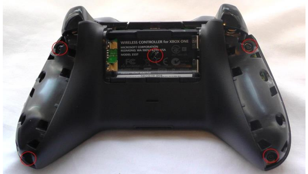
Figure 3. T8 Security Screw Locations
