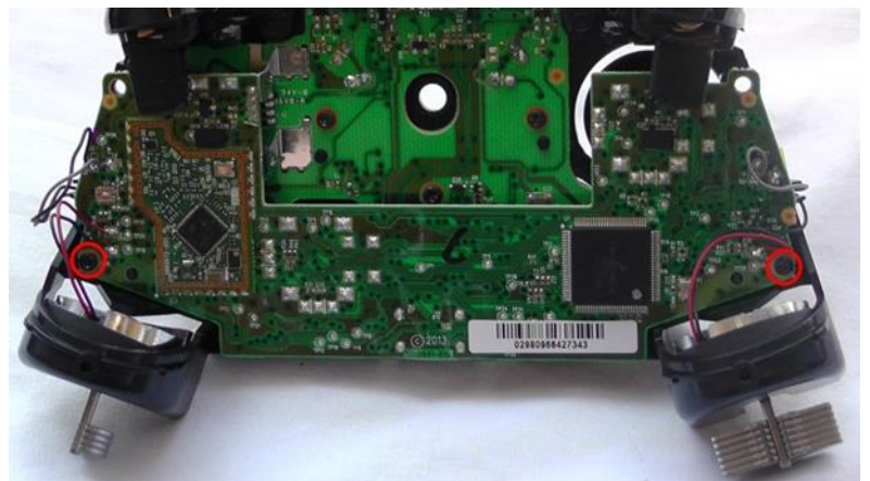
Figure 4. Location of T6 Screws
