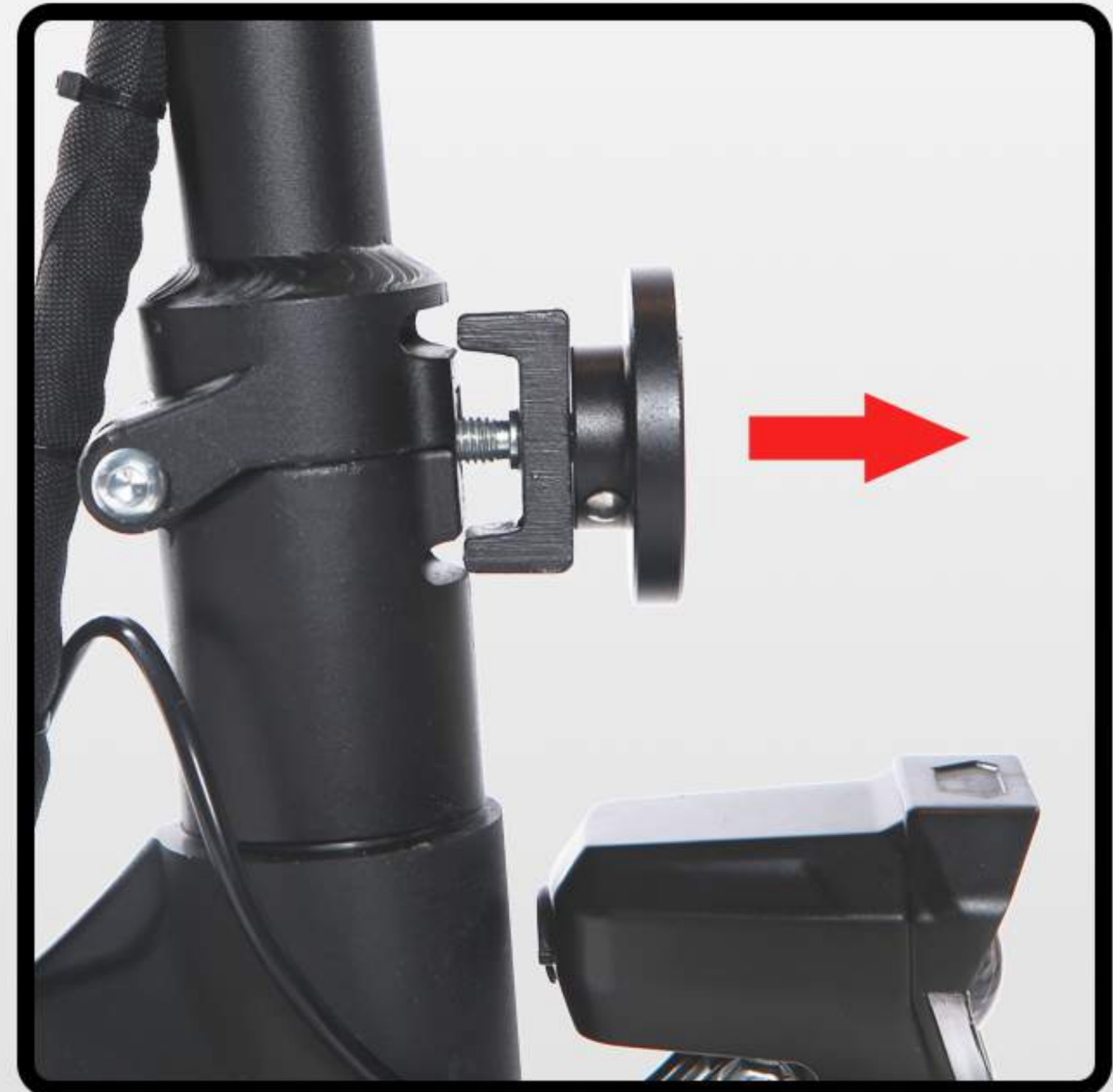
② Keep loosening the folding knob until the L-shaped buckle completely leaves the grooves
