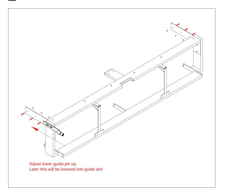
Assemble rotating structure to the front of the metal base using three 10mm L45 machine bolts (F) and two round washers (I) and one washer with flat edge (I).
