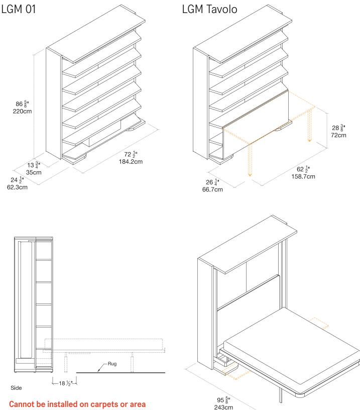
Cannot be installed on carpets or area rugs, if using an area rug it should be placed a minimum of 18 1/2" from front edge of the LGM.
