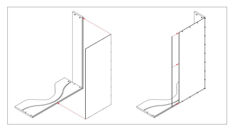
3 Install the second back panel. Do Not Use any Wood Screws Yet. Attach the top to the left side using cam connectors (K).
