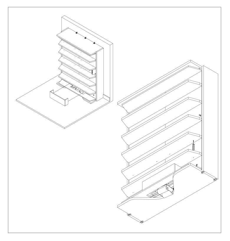
Lift the wooden mattress support onto the metal base. Remove the nuts from the bolts located on the bottom of the springs. Insert the bolt into the slots on the metal base and then tighten nuts onto bolts. Slide the two night stand shelves into the grooves. Note position of the finger pull in drawing.
