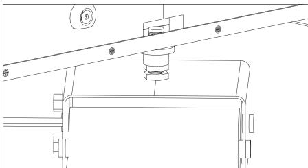
Thread the top guide roller(Code M) into the groove inside the top of the bed structure. 2 and 3. Attach metal support arm to the upper bed structure using brass bolt (Code L) 4. Lower guide pin: Insert the lower roller into the groove on the lower section. After the top roller guide, metal arm and lower pin have been installed, rotate the unit a few times and make any necessary adjustments to the roller, and lower support metal arm.
