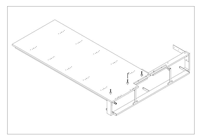
Stand the structure and base upright and install the 2nd panel.
