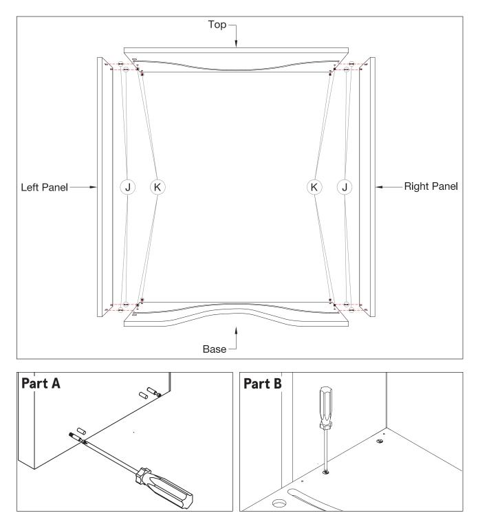
2 Install the left back panel into the bed structure with the groove facing the center. Use Wood Screw 3.5x30 (B) to attach Backpanel. Install the brown spline into the groove. Bed also available with wide vertical sides. Not shown in these instructions.
