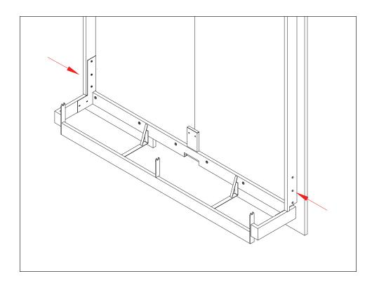
14 Install the top of the rotating unit. Align the brass dowels to the holes in the top. Starting from one side install the 6mm L30 (Code D) machine screws. Gradually tighten the screws until the top pulls tight against the front panels. Now tighten the 6 bolts (g) and the 6 nuts and bolts from step 13.
