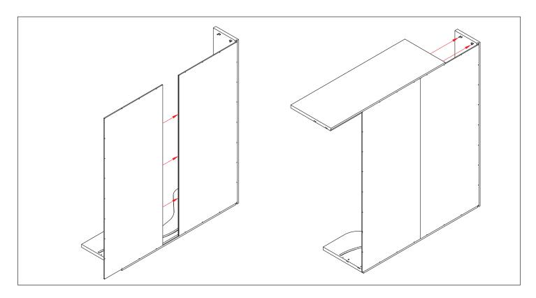
Attach the right vertical side to the bottom and top using cam connectors (K). Install the remaining screws into the back panels using wood screws 3.5 L30 (B).
