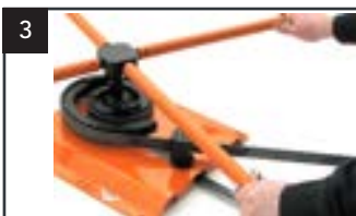
3 Rotate handles clockwise to form scroll to your desired size. Unlock and lift segments to release finished scroll.
