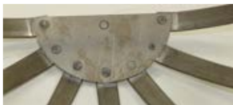
Half Disc connector plate used to make half basket.
