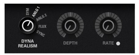
The DYNA REALISM Mode Selector switch sets how much left/right channel, and unit-to-unit variations occur throughout all circuits in the digital model including Mojo, EQ, and Aspect Ratio by choosing component values from the appropriate Virtual Parts Bin. These subtle differences can enhance the depth and width of the stereo image.
