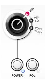
MIX mode allows all processing blocks of the plug to be enabled. This is the default mode.
