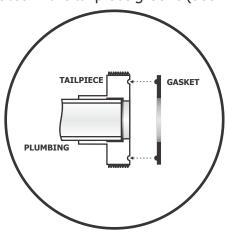
**9 -** You are now ready to install the heater in the open space between the two (2) tailpieces (ensure that the gaskets remain in place). Slide both heater nuts inward toward the center of the heater to expose the mating surfaces of the heater housing. Slide the heater carefully into place between the tailpieces and gaskets and hand-tighten heater nuts. If you use a wrench be careful not to over-tighten, the nuts can crack (see Fig. 25).
