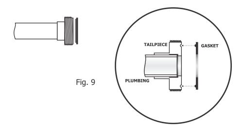
4 - You are now ready to install the heater in the open space where the Heater Ready fitting was located (ensure that the gaskets remain in place). Slide both heater nuts inward toward the center of the heater to expose the mating surfaces of the heater housing. Slide the heater carefully into place between the tailpieces and gaskets and hand-tighten heater nuts. If you use a wrench be careful not to over-tighten, the nuts can crack (see Fig. 10).
