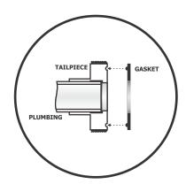
**9 -** You are now ready to install the heater in the open space between the two (2) tailpieces (ensure that the gaskets remain in place). Slide both heater nuts inward toward the center of the heater to expose the mating surfaces of the heater housing. Slide the heater carefully into place between the tailpieces and gaskets and hand-tighten heater nuts. If you use a wrench be careful not to over-tighten, the nuts can crack (see Fig. 19).
