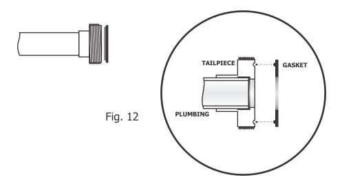
**4 -** You are now ready to install the heater in the open space where the Heater Ready fitting was located (ensure that the gaskets remain in place). Slide both heater nuts inward toward the center of the heater to expose the mating surfaces of the heater housing. Slide the heater carefully into place between the tailpieces and gaskets and hand-tighten heater nuts. If you use a wrench be careful not to over-tighten, the nuts can crack (see Fig. 13).
