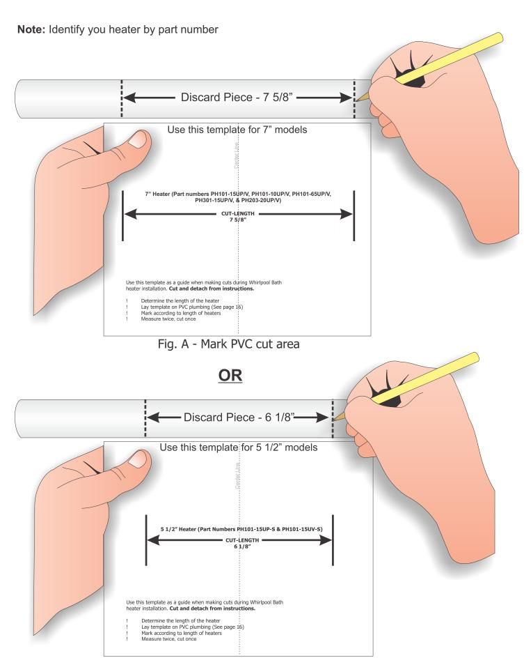
Fig. B - Mark PVC cut area
