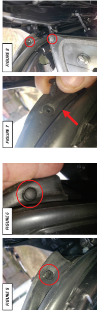
4. Remove the side mirror (FIG 5).
