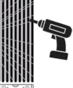
Install the acoustic panels with screws or adhesive through the polyester on wall or ceiling.Use 15 screws to each panel.Form work shall be distanced by 60mm.Always use screws when mounted on ceilings.
