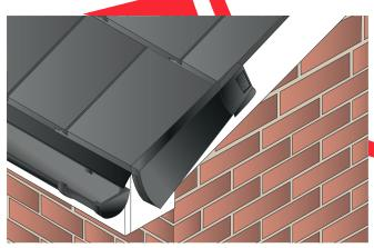
4 Slide the first verge unit over the tile at the eaves, and into the starter kit, fitting it under the head laps to ensure the unit is firmly held in place. Screw fix the unit through the top grid into the batten.
