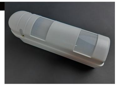
By using the two infrared sensors in «AND» mode (one with view parallel to the ground and the other one tilted downward), the «Pet Immune» mode can be enabled. In this mode, the movement of an animal passing below the installation height of the detector is not detected.
