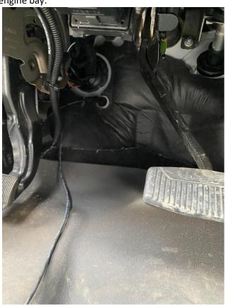
2. Locate the harness in the engine bay and pull it through with out causing tension. You will now put the YELLOW and White wire in to the connector like so;
