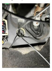
2. Locate the harness in the engine bay and pull through some of the harness with out causing tension.
