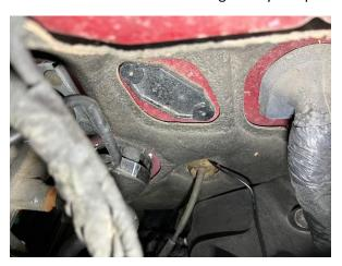
3. Locate the CCV Conncetor and disconnect it by releasing the sliding red locking tab.
