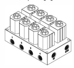
IN Ports: Air supply from air tank. (we always recommend the use of a water trap between air tank and valve manifold)
