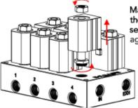
Make the internal cleaning of the valve with the aid of a deseize and assemble the set again.
