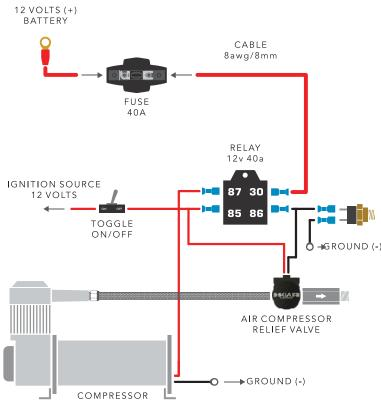
The air compressor relief valve installation should be done by a professional. In pneumatic installation, the relief valve must be between the electric compressor and check valve. In the electrical installation, the valve must be connected to relays pins 85 and 86.
