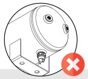
We do not indicate the installation of the pressure switch with the thread facing upwards, as this way, the internal oxidation process is constant, which can cause a malfunction of the product.
