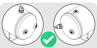
The pressure switch must **always** be installed with the thread facing downwards or in a horizontal position.
