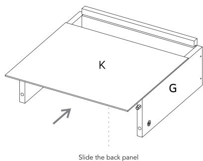
Slide the back panel inside the grooves.
