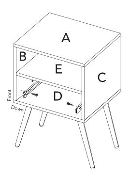
The wheel should go towards the front edge of the panel and facing down, like this:
