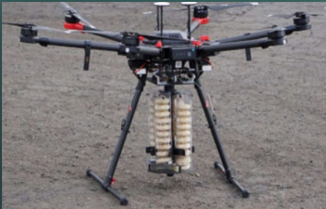
Example of microsensors attached to an unmanned aerial vehicle for strategic placement. (DTRA JSTO photo)
