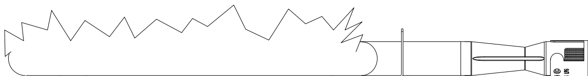
Poor Combustion: wavy, yellow flames-too little air
