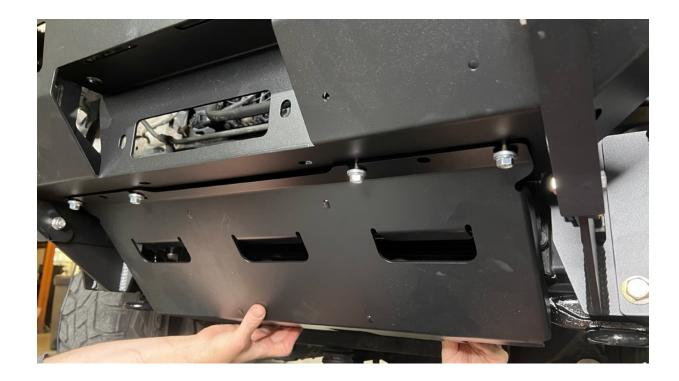
1DA The bolt holes on the tie-in skid are slotted to ease installation. In step 4A we left the bolts under the center section loose, slide the tie-in skid udner those bolts as shown. You'll may need to remove the forward most bolts on your front skid to get the tie-in skid on
