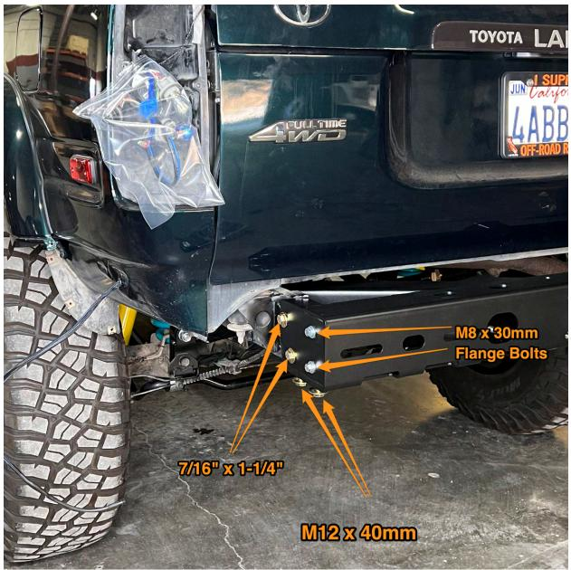
Next Make sure to install the wing stiffeners (triangular pieces with 3 weld nuts), the trailer plug, and lights into the bumper wings before sliding the bumper wings onto the frame and cross member. The M12 x 40mm bolts that go under the frame in the above photo get installed AFTER the bumper wings get installed
