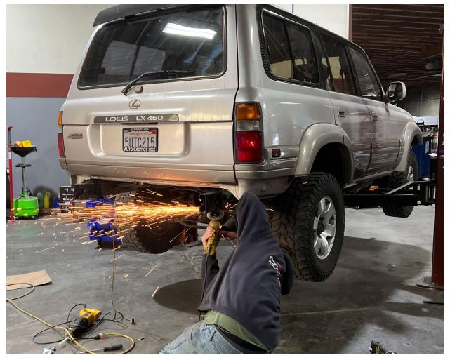
Make sure you get these nut plates inside the frame and start the threads before attempting to put the new cross member over the frame
