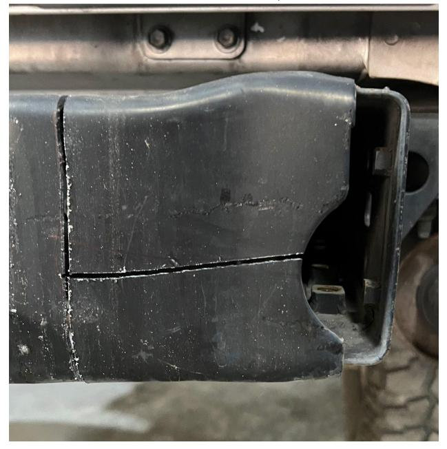
You want to score the welds so we can snap off the crossmember without cutting the primary frame rails
