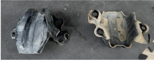
**2B** Remove the two metal bowlshaped covers on the front differential.
