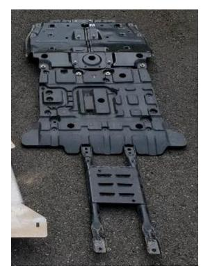
2A Remove two front plates, front plate cross member, large plastic engine cover (with oil access door), and metal "H" transmission plate. There is a combination of 10mm and 12mm hex bolts throughout.
