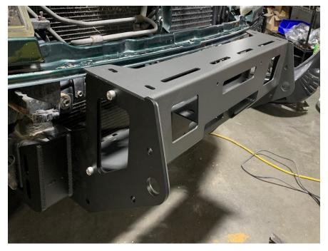
Now mount the center section of the bumper on top of the frame brackets using the 3/8" socket head bolts in the locations shown. Install the bolts from the outside with no washer and a washer and nut on the inside to hold it in place. If needed you can install the top plates onto the center section with the shorter 3/8" bolts to give the center section more area to hold.
