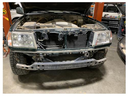
To remove the factory bumper you will need to first remove the grill by unscrewing the three phillips screws and undoing the two tabs at the bottom. Next remove the three clips and 6 bolts (10mm) attaching the bumper to the body. Unplug the fog lights and the bumper should now be free.
