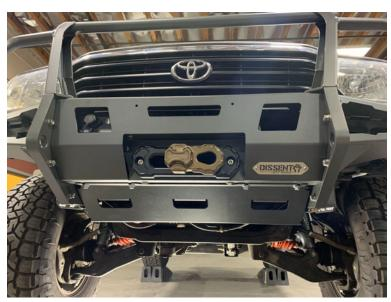
Install the tie in skid using the separate hardware kit with M8 bolts and nut plates for inside the center section.
