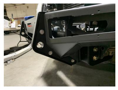
Set each wing into place, and install the recovery point caps with the longer 3/8" stainless steel bolts. These bolts will also mount from the outside with washers on each side and 3/8" stainless nut.
