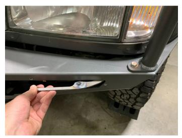
If you purchased the bull bar for your front bumper, you can use the supplied nut plate to make the wing portion easier to bolt on.
