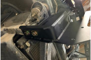
Mount the frame brackets with the supplied M14 bolts and large washers with the risers toward the inside of the frame. Tighten to finger tight so that you can make any adjustments needed later.
