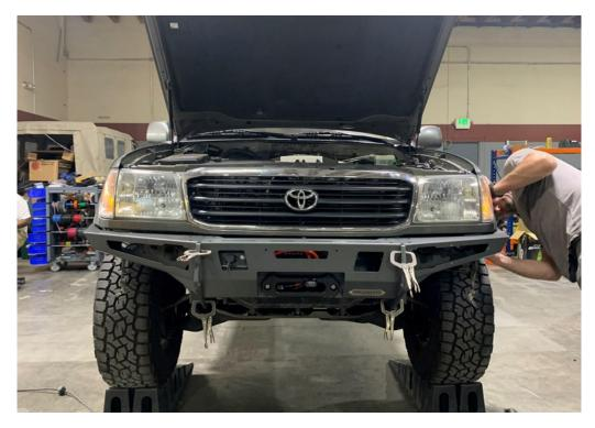
Using the socket head bolts to position, you will now temporarily clamp both wings in place to align the bumper. Move the frame brackets forward or back to get a 1/8" - 3/16" gap between the center of the bumper and the lower grill valance. By using the supplied shims in between the bottom of the frame and the frame brackets, you want a minimum of ½" gap between the wings and fender. It is not uncommon to use a different amount per side to get the bumper level.
