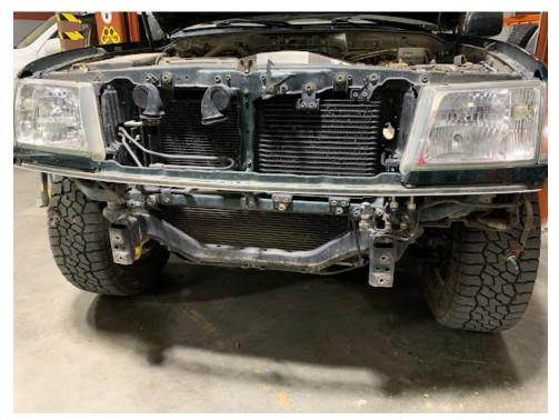
Unbolt the "crash bar" (4 14mm bolts) and remove any factory or aftermarket tow hooks/recovery points that are bolted to the bottom of the frame.
