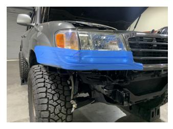
You should now paint the areas on the frame that you have modified to prevent corrosion. Also depending on the condition, you may want to also paint the valence under the grill and headlight area.
