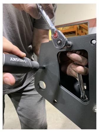
You can now begin reassembling the bumper following the previous steps. Before tightening the socket head bolts to mount the center section to the frame brackets, use a screwdriver to perfectly align all of the recovery point cap holes.
