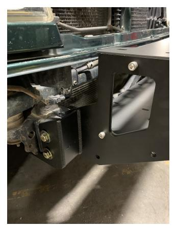
Install the 4" through bolts from the outside of the frame brackets with washers on each side and a ½" nut on the inside.
