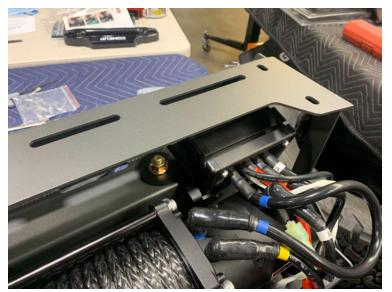
If you purchased a ComeUp winch from us, you can use the supplied bracket to relocate the control box to inside the center section as shown.
