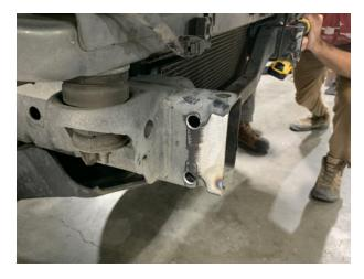
Using a good step bit, you will drill %" holes on the inside/outside and top/bottom of both sides of the frame. It's a good idea to make your holes as close to the top and bottom of the frame for the most strength and level from inside to outside so that the through bolt installs correctly.
