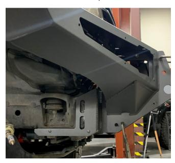
Once you are satisfied with the alignment and placement of the bumper, mark the outline of all four holes (inside and outside) on both frame brackets.
