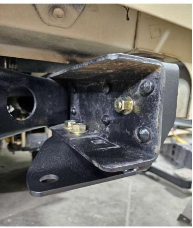
Temporarily install hitch to rear crossmember to mark and drill two new holes. For the 60 series hitch you'll install the bottom bolts where the flange goes under the crossmember.
