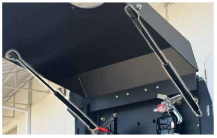
The bottom tray installs as depicted below. A UHMW pad should come pre-installed to act as a latch-catch.
