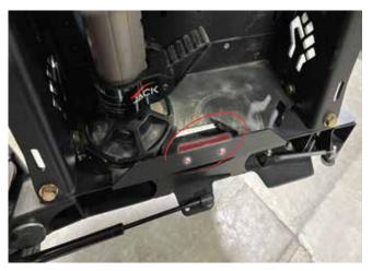
The latch installs using its included hardware. Ensure the latch is installed without the screw on the latch portion, this screw should be already removed prior to installation. Two pieces of weatherstrip adhere to the bottom of the door as highlighted below:
