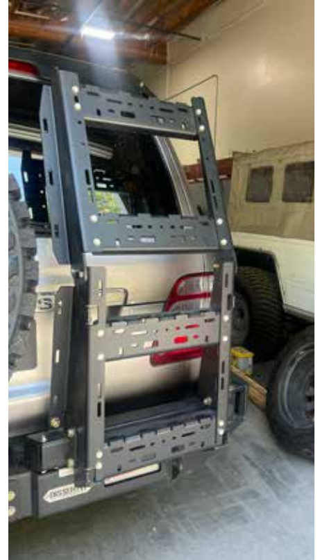
(Ladder Rungs install using the provided bolts as shown)
