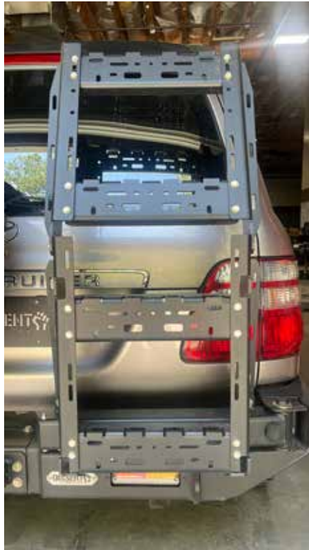
(Ladder Rungs install using the provided bolts as shown)
