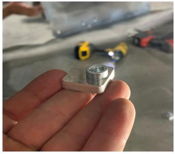
Now you can mount the rear skid plate above the middle skid and use the small offset nut plates for the 4 rear most holes with the regular flange bolts and thick washers. Note the orientation of the nut plates when installing is just like in the picture with the pem nut on top. The remaining counter sink bolts and washers can be installed at the intersection of the middle and rear skid.
