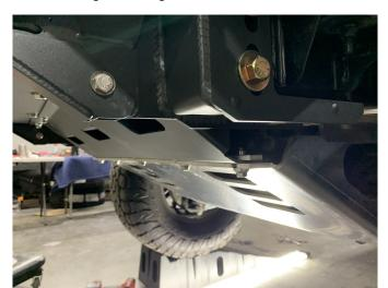
If you have purchased/installed a Dissent front bumper your tie in skid plate will mount using the same bolts as the front skid plate and the included large pem nut plates for the 2 outside holes.
