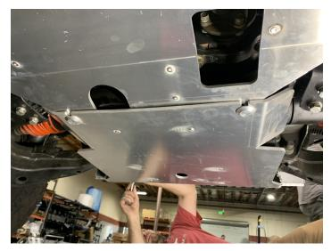
Install the front skid plate beginning with the rear below the middle skid and use the remaining regular flange bolts and washers to install the front, sides and middle hole locations.
