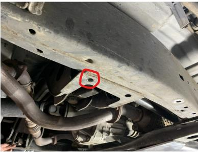
Using a step bit, enlarge the rear most mounting holes on both sides near the torsion bar adjustment bolt to roughly the same size as the one opposite of it.
