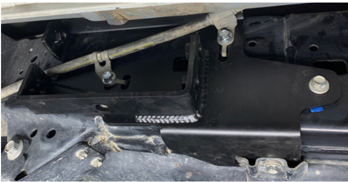
Rear bracket: four bolts along side of frame, one underneath
