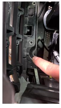
fashion a new way to secure the bottom of the grill using the three clips we removed in step 5. Place the grill where it should go
