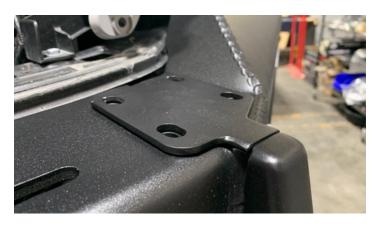
recovery point cap on, thread the bolts (with washers on both sides) from the outside in making it finger tight to start.
