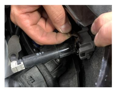
13. Remove the headlight washers themselves from the inside of the bumper. First remove the metal retaining clip, this allows the gray body to slide back. Then, from the front of the bumper, squeeze the tabs that hold the washers to the bumper and they should come free. 14. We'll be reusing the headlight washers and the fog light wiring harness, so free the washer water lines and wiring harness from the factory bumper and set them aside.
