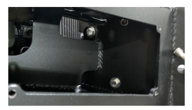
center while you thread two 3/8" x 1-1/4 bolts w/ washers through and backed by a washer and 3/8" nut. Torque to 25-30lb/ft.
