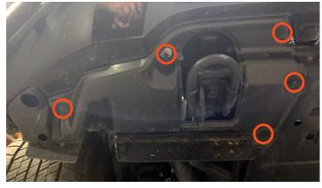
10. Start to pry the front bumper off where it meets the fender. Carefully loosen the bumper and work the entire bumper off the vehicle.
