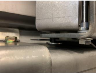
Install the 2 outer 7/16 bolts on the hinge with the swing arm closed. While paying close attention to the uhmw pad, tighten the outer bolts. (We will torque to final spec after checking alignment). Once tight you can tighten the main hinge bolt to where you feel the preload on the bearings.
