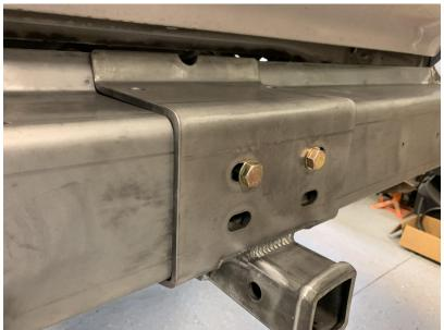
Install the lower hitch bolts loosely.
