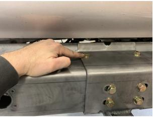
10) Now we will move on to the wing stiffener. Loosely install the three 1/2" bolts on both sides with nuts and washers.
