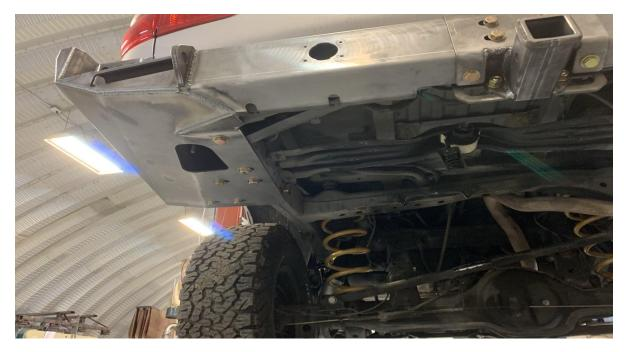
Once installed you can tighten up all bolts. All 1/2", m14 and m12 bolts should be tightened to roughly 95fp.
