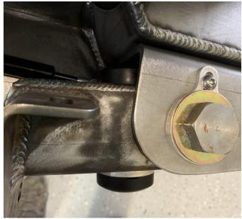
Once the swing arm is installed, aligned and greased we can move onto the tire carrier.
