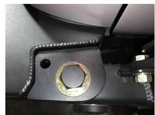
Next you will install the uncoated stainless striker pads with the 1/4x20x3/8 stainless button head bolts.
