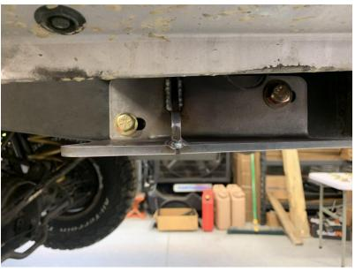
5) Using masking tape, tape on one of the 1/4" hitch spacers to the frame. (Note, on some 03 and up models equipped with the integrated towing cross member these spacers will not be used.
