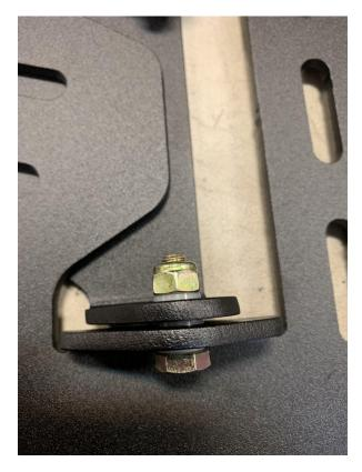
Next install the back plate on the front plate as pictured. (Note the orientation of the bolts and duplicate the photo)
