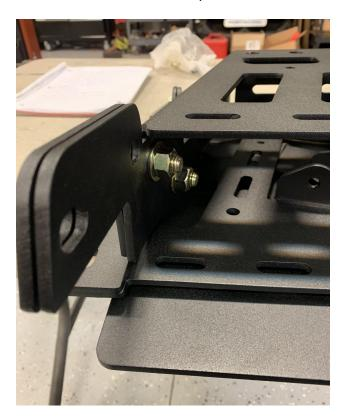
Tighten all bolts and install table/tire assembly onto the swing arm. Adjust tire to desired height and angle and tighten bolts.
