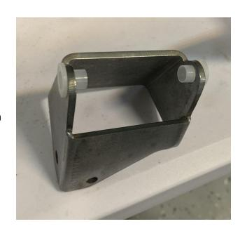
Install the 5/16 stainless bolt from the bottom of the swing arm up. (Nut will be on top) use anti seize on threads!
