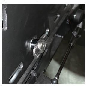
Install the table with nylon washers as shown below.
