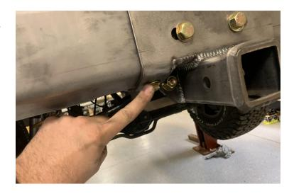
Next, the back 1/4" spacer and back plate can be installed along with the 4" through bolts. Install all hitch bolts loosely.
