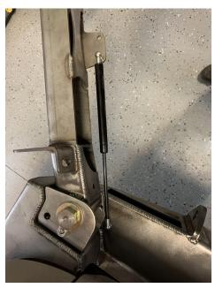
Once the gas strut is in place, install the 1" bump stop on the inside of the swing arm and the smaller bump stop on the outside.
