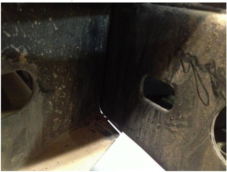
Now, bend that piece back and out of the way, take the sawzall and cut as close to the frame as possible, you will only need to cut part way through and then it will break off
