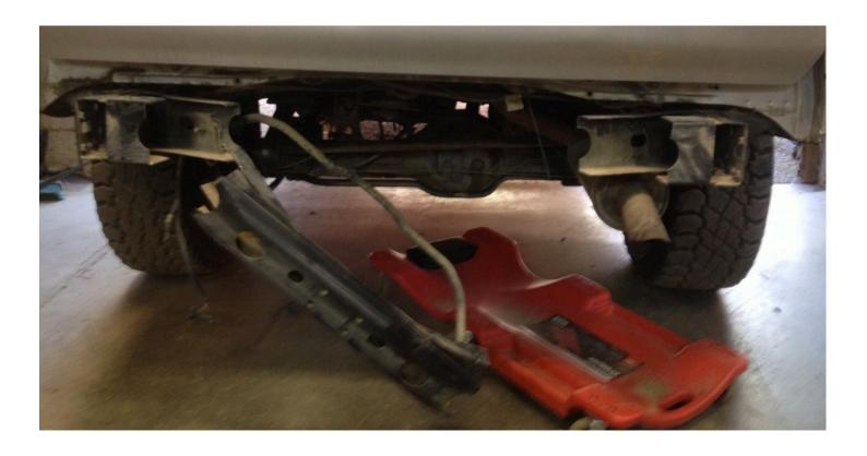
Next, you will cut the top and bottom of the piece attached to the frame, cut as close to the frame as possible.
