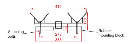
DISTANCE BETWEEN BOLT HOLES FOR DEPTH = 276MM (276 CM)
