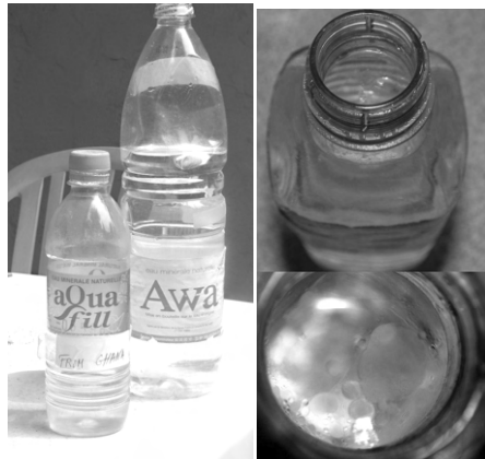
Unopened water bottles from Africa develop oil slicks at the surface in 3 to 6 weeks, if left undisturbed.
