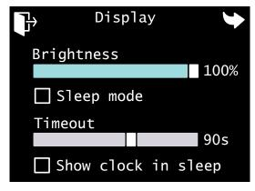
Screen five allows you to adjust the brightness of the panel and whether the panel goes into sleep mode.
