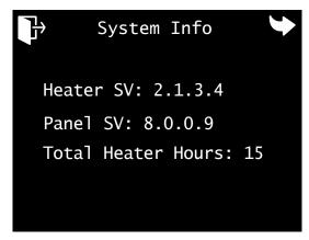
Screen four gives the software versions for both the heater and the control panel and the total hours that the heater unit has been running.
