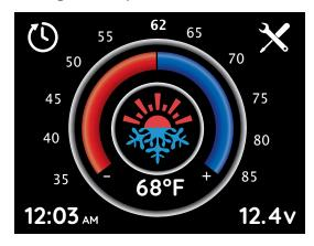
Set the temperature by touching the temperature dial and rotating it to the preferred setting or by touching the plus or minus buttons below the dial. To finalize, touch the logo inside the dial.
