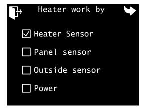
Screen one in settings allows you to choose which sensors you prefer the heater to work by. The system has three possible sensors:
