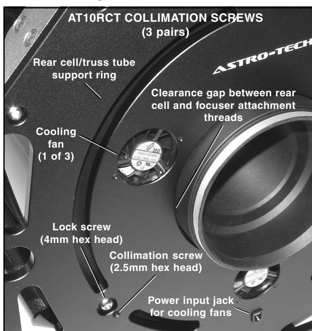
and the focuser to let you adjust the tilt of the collimation ring to zero out any tilt in your focuser during final scope collimation.
