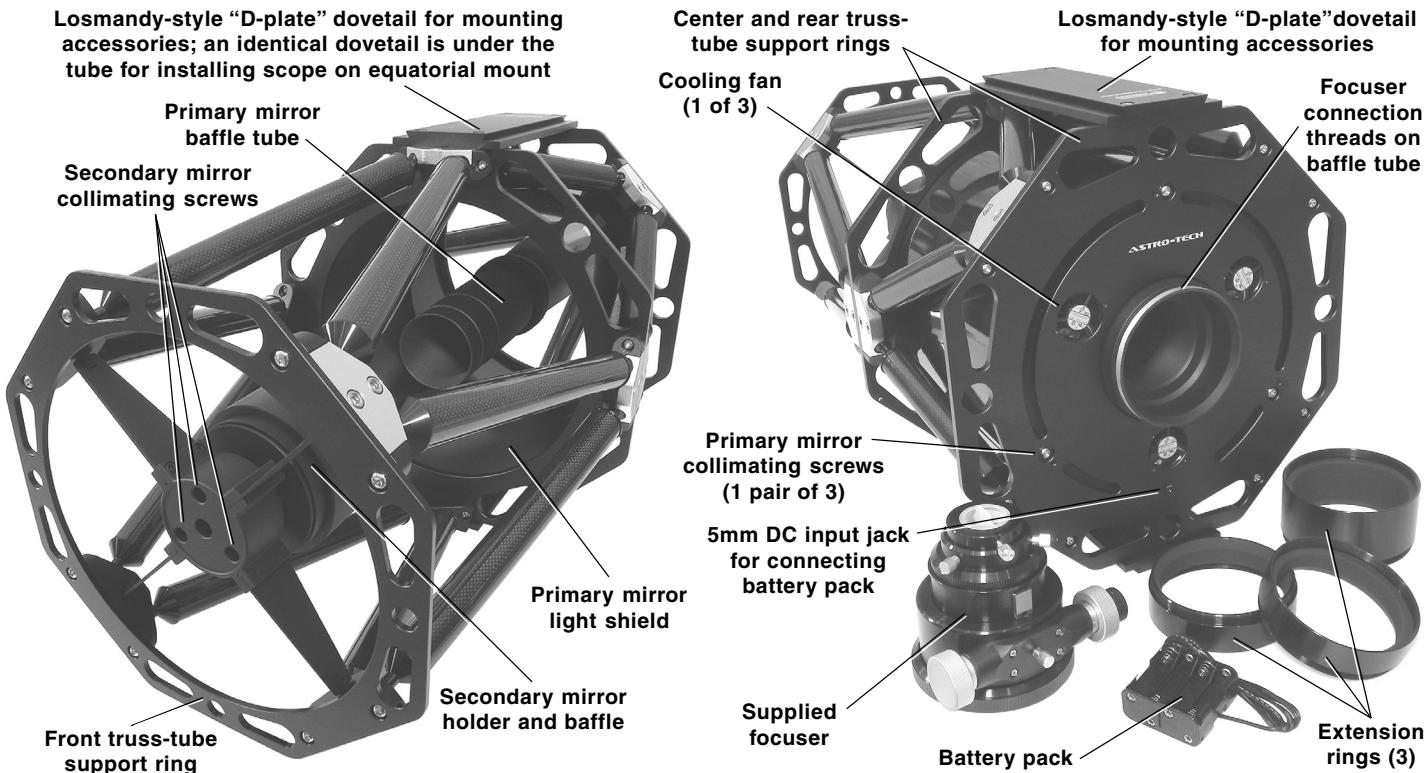
**Focuser:** The AT10RCT comes with a dual-speed linear bearing 3" Crayford focuser for use with light imaging trains (such as a DSLR body only). However, a very heavy multi-component imaging train would probably require an upgrade to a rack-and-pinion focuser to support its extra weight. Alternatively, you may already have a premium focuser you use on another scope that you would like to use for imaging, or you may want to install a robo-focus for use at a remote observatory.
