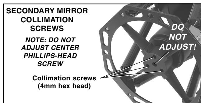
**Caution:** Do not adjust the recessed Phillips-head screw in the center of the secondary holder, as this will change the primary to secondary mirror spacing and degrade image performance.
