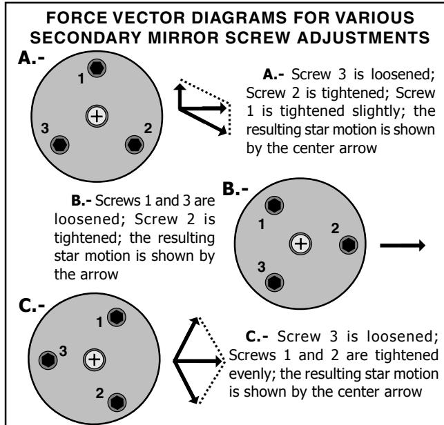
Repeat the collimation procedure several times, using successively higher power eyepieces, until you are sure the collimation is exact. Finally, after the final adjustments have been made, make sure that all of the collimating screws are snugged down tightly and evenly to ensure that the collimation will hold for many trips out into the field.
