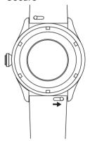
Release the peg to secure the strap into the lugs. You may need to wriggle the strap until the pin falls into place. When it does, you should hear a 'clicking' sound.
