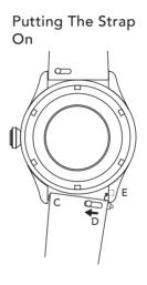
Position the pin that is opposite to the peg into its relevant hole on the watch's lug (C). Once in place, pull the peg to the left side (D) and align the remaining pin with its hole in the lug (E). Release Peg To Secure
