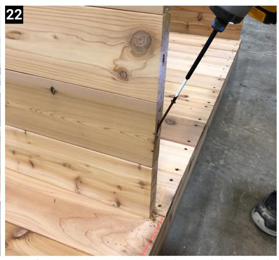
Using 4" screws and using the existing holes, attach the other side of the front wall together.
