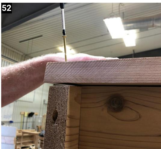
Put flush to the back and secure down with a couple 3" screws.
