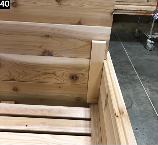
Then attach to the front and back wall with 3" screws.
