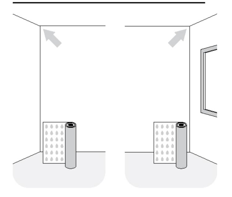
In order to stick the print evenly, you can measure and draw vertical lines on the wall approx. 2 cm narrower than the width of
