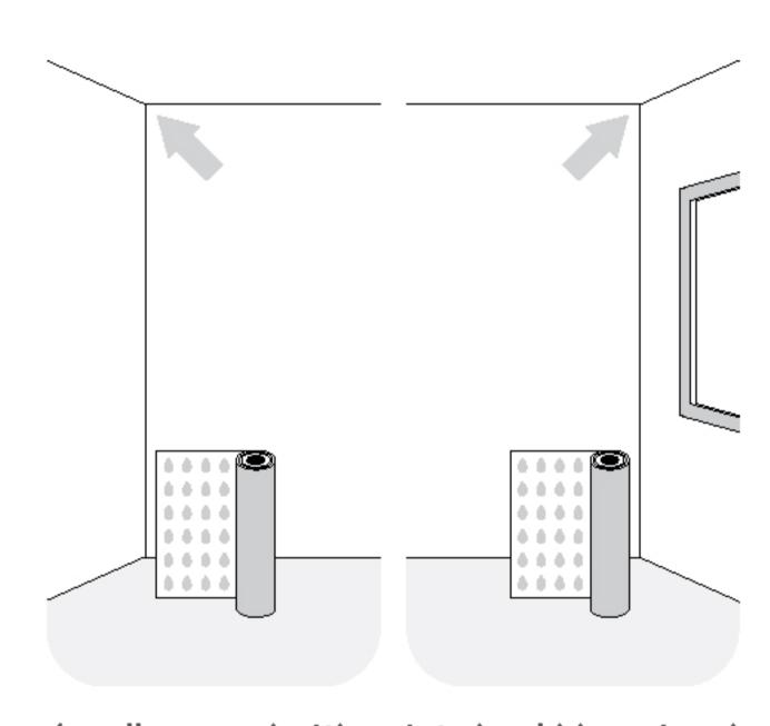
A wall covered with paint should be primed once, and in the case of a thick layer of paint (e.g. silicone, washable), rub with sandpaper (to increase the adhesion of the adhesive to the substrate) and degrease.
