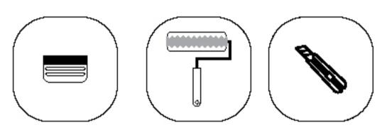
A fresh wall - covered with gypsum plaster, plasterboard or other absorbent building materials, must be primed twice with deeply penetrating primer at least 24 hours before application. It is necessary to ensure that the primer soaks into the substrate and does not leave a layer on the surface that could weaken the adhesive.
