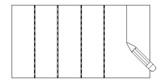
In order to stick the print evenly, you can measure and draw vertical lines on the wall approx. 2 cm narrower than the width of the wallpaper or use a laser level.
