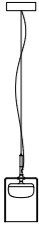
S1 Ceiling Rose Ø 160 mm H 40 mm Cable 2000 mm Diffuser Ø 180 mm H 240 mm
