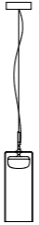
S5 Ceiling Rose Ø 160 mm H 40 mm Cable 2000 mm Diffuser Ø 180 mm H 450 mm
