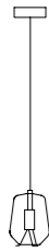
S1 Ceiling Rose Ø 160 mm Ceiling Rose LED DIMM Ø 200 mm Cable 3000 mm Diffuser Ø 200 mm H 285 mm
