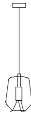
S3 Ceiling Rose Ø 160 mm Ceiling Rose LED DIMM Ø 200 mm Cable 3000 mm Diffuser Ø 320 mm H 450 mm
